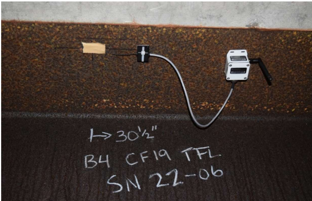
Figure 1. Sample Wireless Sensor (Strain Gage) with a Transmitter
